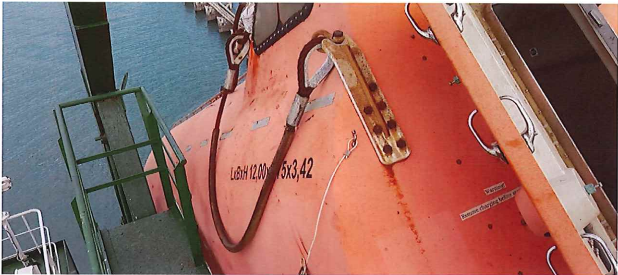
Figure 1. Lifting sling encased in plastic sheathing
