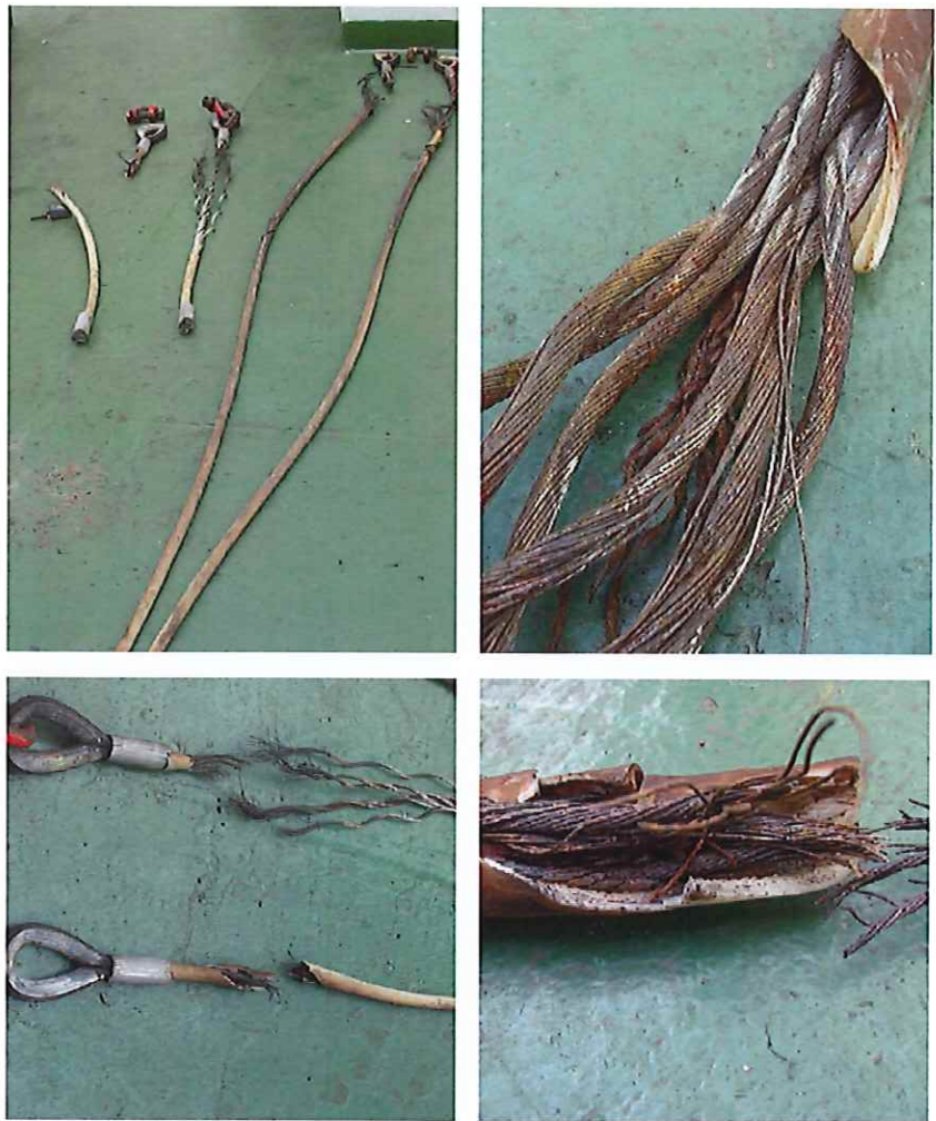
Figure 3. Lifting slings parted due to undetected corrosion.
