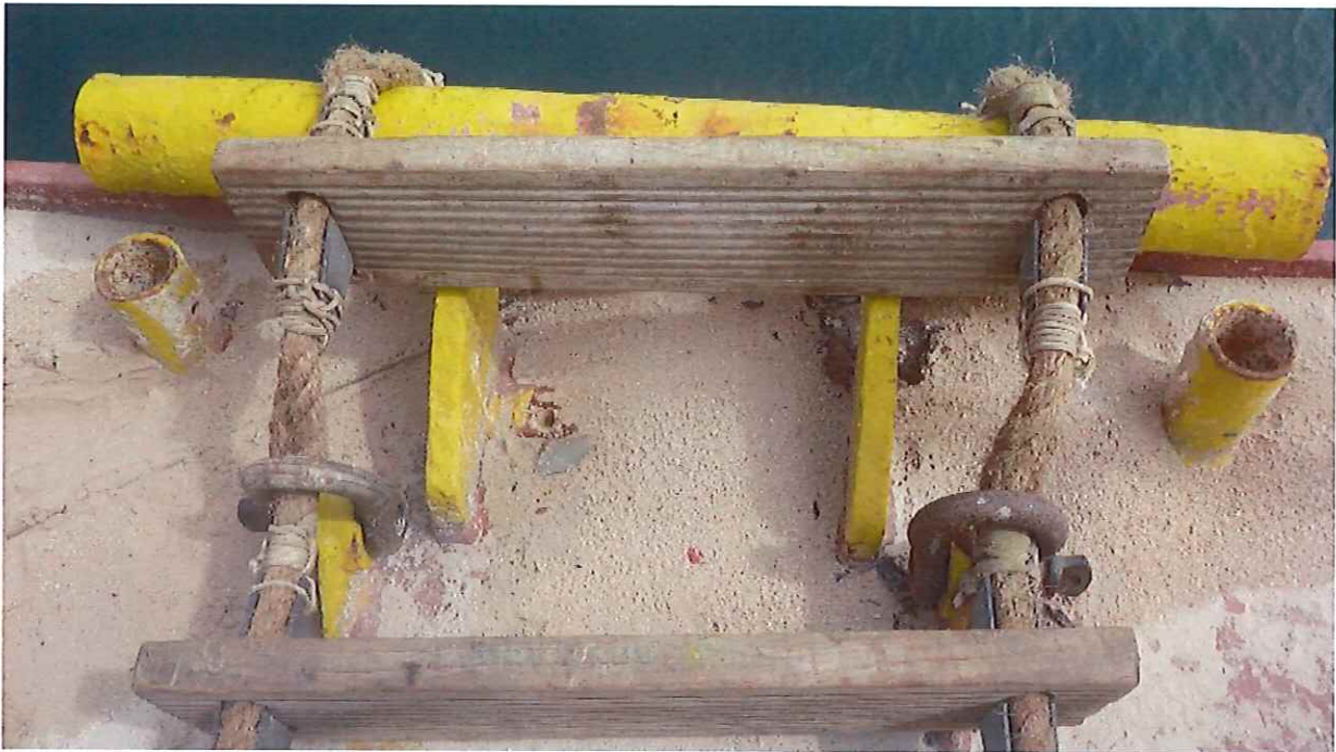
Figure 1. Pilot ladder incorrectly secured to the deck using D-shackles to choke the side ropes.
